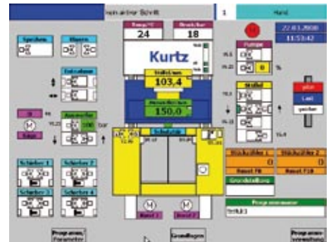
Visualization with large color screen, controlled via protected keyboard. Trimming recipes saved directly on Secure Digital Memory Cards.
