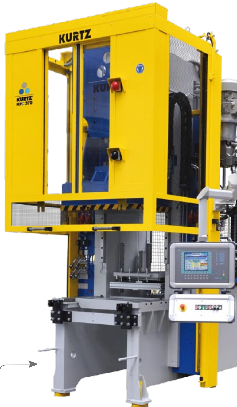
KPC 370: C-Press frame with a 37 ton closing force with opened press guard for simple mould change
