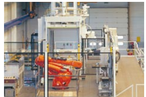
Automatic casting solution with robots, safety guards, burr removal including CE-certification for the entire cell.
