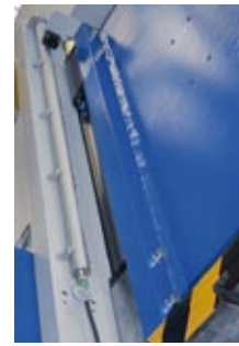
Position measuring system for clamping platen.
