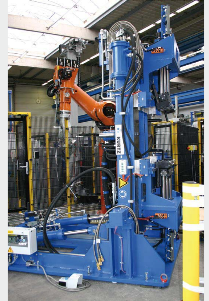
Tiltable gravity casting machine, tilted by 90°, servo-hydraulic tilting motion, tilting angle of up to 110° possible
