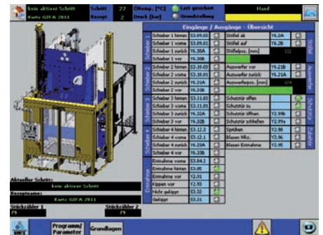
Visualization with large color screen, controlled via protected keyboard. Trimming recipes can be saved directly on Secure Digital Memory Cards.
