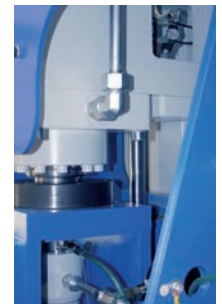
Clamping platen safety device. Clamping platen connection with position measuring device.
